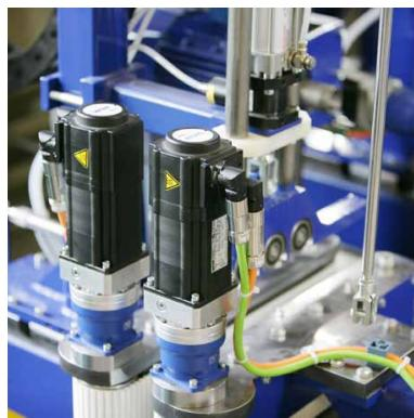
The servo motors are equipped with commercially available connectors as standard.
